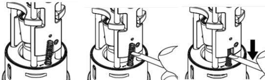
6. Loosen the grip adapter screw with the 0.9mm hex key from the *Precision tool kit No. 90*.
