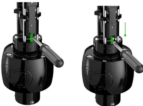
6. Remove the Stay up spring No. 24 on the side "1", by pressing down the spring with the small flat screwdriver. Put one corner of the screwdriver between the fourth and fifth coil and press the spring down as straight as possible until it comes clear and can be taken out. Keep your thumb over it so it doesn't spring away.
