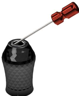
8. Tighten the screw with the 0.9 Hex key (red) from the *Precision tool kit No. 90*. Make sure the key engages in the screw properly before tightening so the screw is not damaged. Tighten medium hard and make sure you don't bend to the side which can damage the key or screw.
