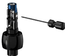
4. Place the Blue drive magnet in the slider. Check that the magnet holder is parallel to the slider before tightening the screw. Mis-alignment can damage the thread. Fasten the magnet holder with the screw.
