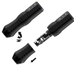
1. Remove the grip, Hold the tattoo machine and turn the grip 30° counterclockwise to remove the grip from the tattoo machine.
