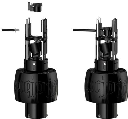
5. Mount the Give adapter No. 148 (included in *Conversion kit No. 110*) on the side of un-marked side, make sure the screw goes smooth into the Give adapter, if not back the screw out, align and try again so that the thread is not damaged. Tighten gently.
