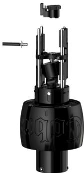
3. Mount the Counterweight on the Slide on the side marked "1". When correct mounted, the counterweight and the spring should both be located on the "1" side of the machine.
